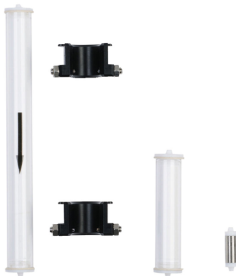
Figure 1: SMART, column adapters, Aluminium oxide, and Carbon column as used for the experiments
